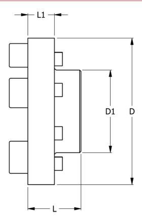
D = 440 D1 = 265 L = 180 L1 = 64 Max bore = 160 Torque (N m) = 13500
